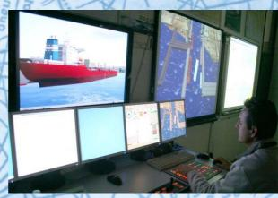
Virtual Bridge and Smartboards Used for Guided Simulation Display
